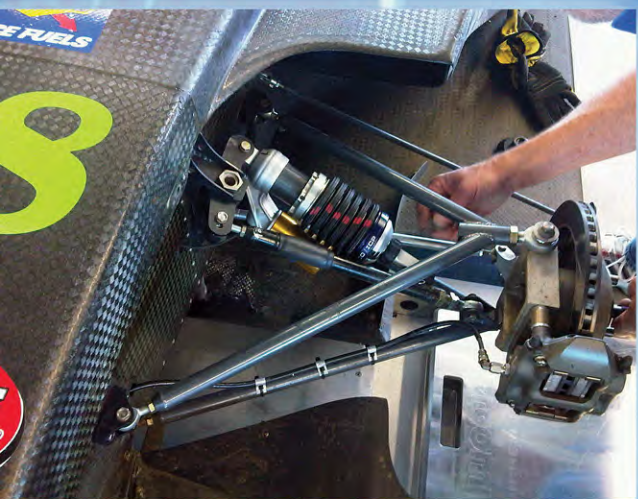
Carbon-Composite Bellows Spring utilized in place of traditional 2" ID x 4" free length steel compression spring.
