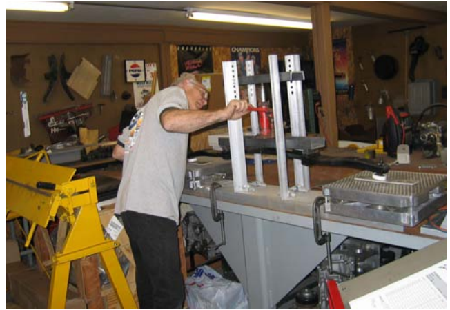
Danny Kellermeyer tests the "street" version of the Composite Leaf Spring on his test stand
